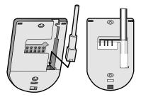
Align the two holes of the case-rear to the holes of the plastic anchors, and then fasten the screwtappings (BH M3 X 30).
